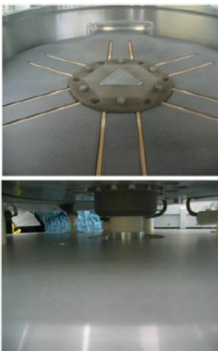
Chamber after 50K Wafers Processed
