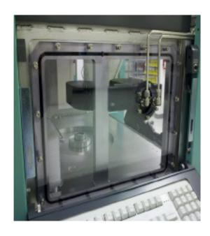
The Enhanced View Port Window upgrade reduces the chance for wafer scrap attributed to incorrect C1 cool station and robot setup and promotes an optimal means for troubleshooting system wafer handling issues.
