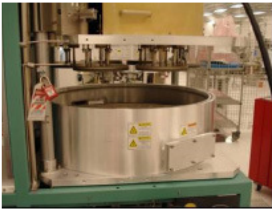
C1 Hoist Lock Assembly Installed
